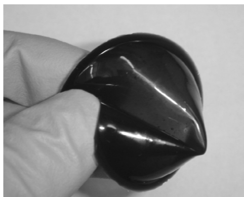
Figure 6. Digital image of 3-trihydroxysilyl-1-propane-sulfonic acid/bis[(3-methyldimethoxy-silyl)propyl]-propylene oxide/bis(triethoxysilyl)octane (A/B/C) membrane containing 2% (w/w) poly-phthalocyanine (polyPc).
